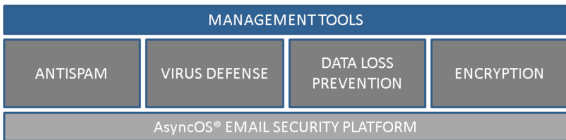
Figure 2. Cisco Email Security Appliance Elements
